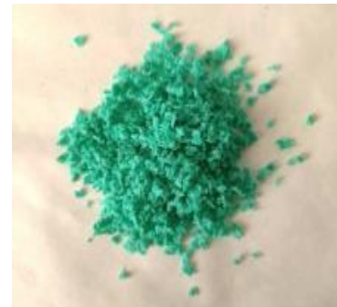
DENSIFIED PP NET AFTER MILLING PROCESS
