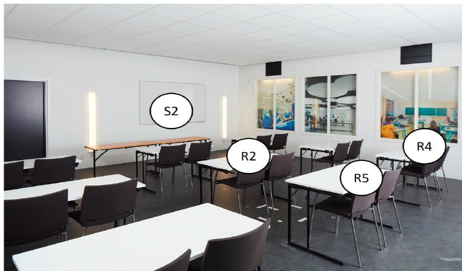
Figure 18 One source / speech position, S2, three receiver positions, R2, R4 and R5, used in the listening test.
